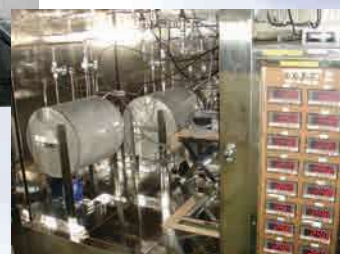
Actual gas flow rate measurement facility
